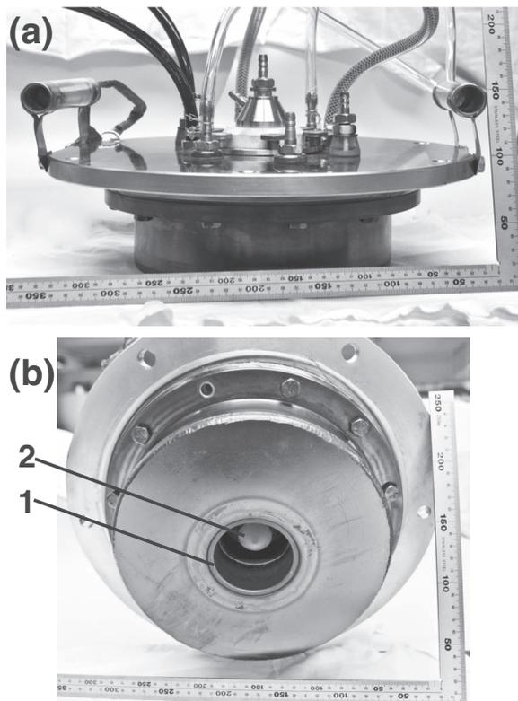
FIG. 1. (a) Photo of sputter enhanced ion-plasma source; (b) bottom source view with 1 – exit aperture (diam. – 60 mm), 2 – sputtering target.
