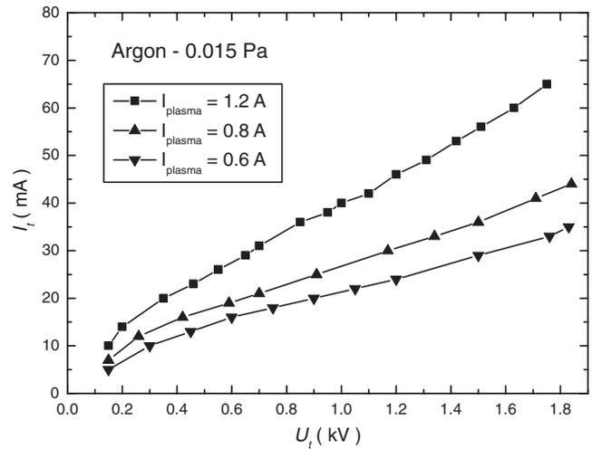
FIG. 4. Titanium target ion current  $I_t$  as a function of sputtering voltage  $U_t$  for the different plasma currents at working pressure of Ar gas 0.015 Pa.
