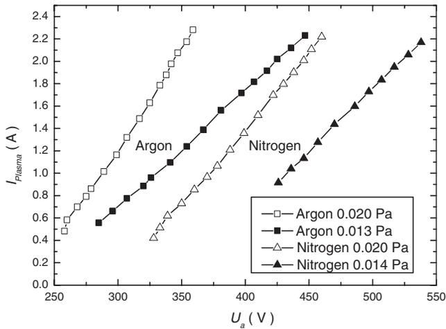
FIG. 3. Typical current-voltage characteristics of low pressure plasma in the source discharge chamber for argon and nitrogen gases at different working pressures.
