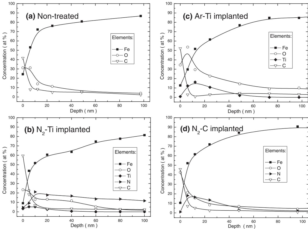
FIG. 8. Surface layer elements depth profiles obtained with the XPS analysis data for the  $\alpha$ -Fe test pieces for (a) – not treated initial condition, (b) – N<sub>2</sub>-Ti ion implanted, (c) – Ar-Ti ion implanted, (d) – N<sub>2</sub>-C ion implanted.
