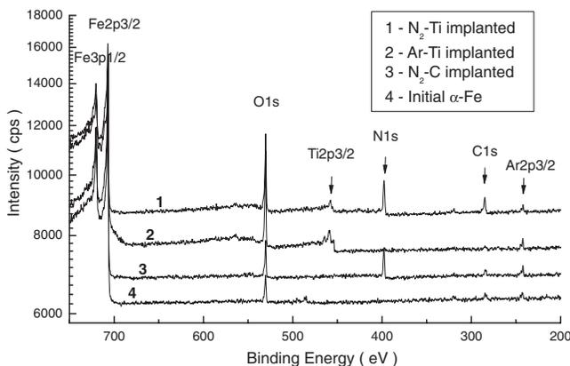
FIG. 7. XPS spectra obtained for  $\alpha$ -Fe test pieces after Ar sputtering to the depth  $\sim 10 \text{ nm}$ . (1) – N<sub>2</sub>-Ti ion implanted, (2) – Ar-Ti ion implanted, (3) – N<sub>2</sub>-C ion implanted. (4) – non-treated initial condition.
