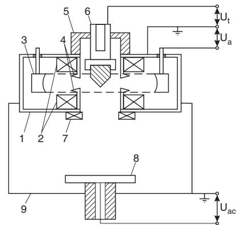
FIG. 2. Schema of the experimental setup equipped with the sputter enhanced ion-plasma source. 1 – water-cooled source body; 2 – permanent ring-shape magnets; 3 – water-cooled ring-shape anode; 4 – top and bottom discharge cathodes; 5 – ceramic insulator; 6 – sputtering target unit; 7 – plasma stabilizing permanent magnet; 8 – accelerating electrode; 9 – vacuum chamber;  $U_a$  – plasma discharge voltage;  $U_t$  – sputtering target bias voltage;  $U_{ac}$  – accelerating voltage.
