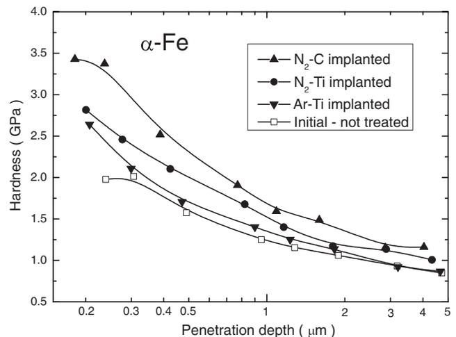
FIG. 9. Dynamic nanoindentation hardness as a function of indenter penetration depth for the initial and mixed beam ion implanted  $\alpha$ -Fe test pieces.
