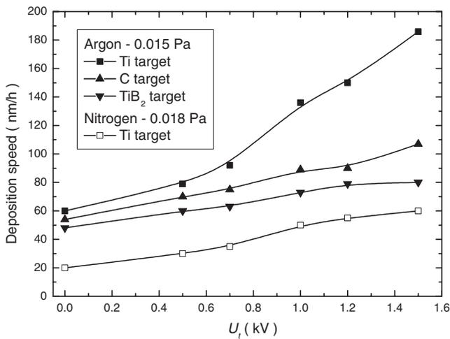
FIG. 5. Coating deposition speed as a function of target bias voltage  $U_t$  for titanium, carbon, and  $\text{TiB}_2$  targets for the case of  $I_{\text{plasma}} \sim 1$  A and  $U_{\text{ac}} = 0$  kV for argon and nitrogen gases.
